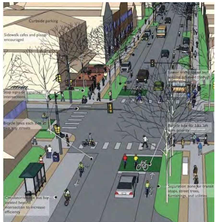
The many functions and components of a street (Credit: Project for Public Spaces)
