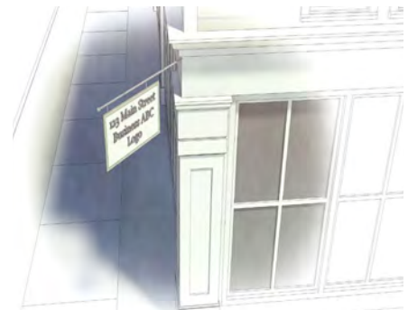
Projecting signs located at building corners where they do not meet perpendicular to the building facade.
